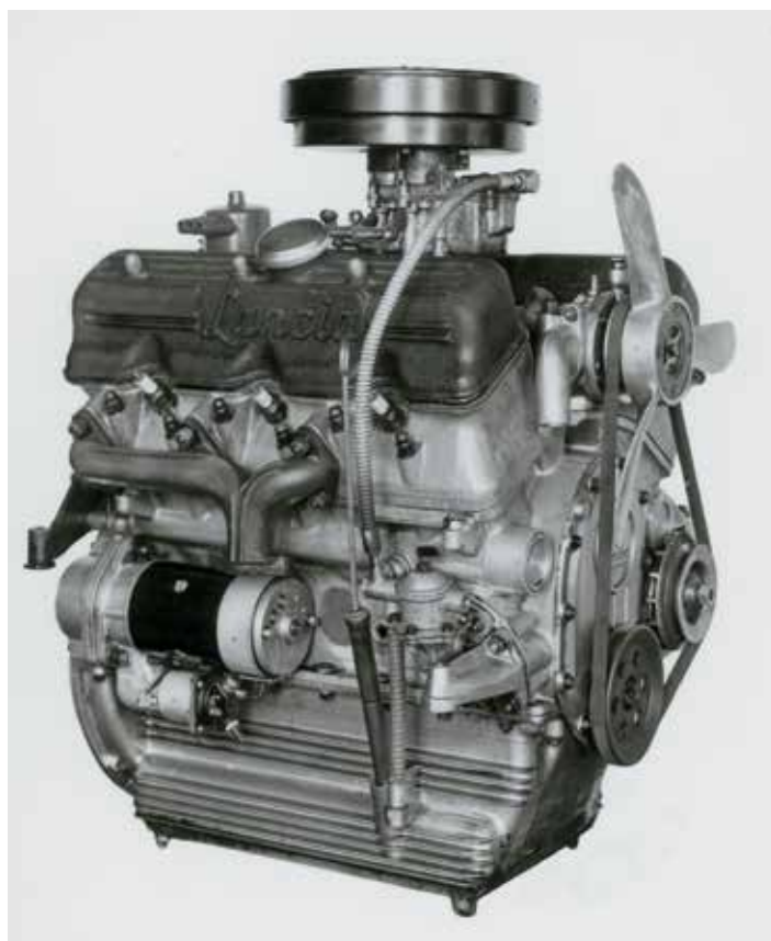
ABOVE Aurelia motor for the s.2 B20 of 1952, identifiable by notches in the valve covers for the spark plugs and two Weber single-choke carburetors. (Centro Storico Fiat)
