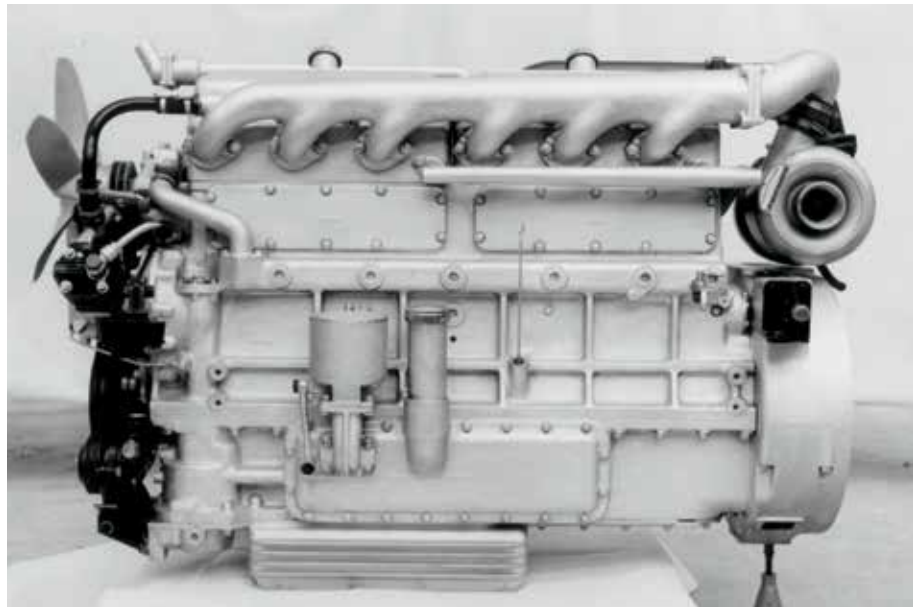
Esagamma engines, the naturally aspirated horizontal version and a turbocharged vertical configuration, which was not put into production. (De Virgilio Archive)
